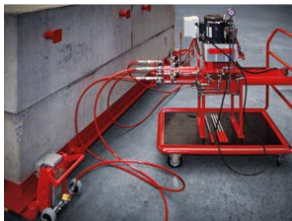
Hydraulic Pressure blocks JD 40 E+ VS in action
