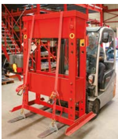
Secure loads with forklift clamps and tension belts
