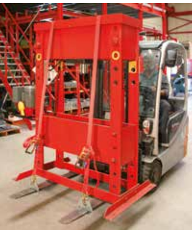
Secure loads with forklift clamps and tension belts
